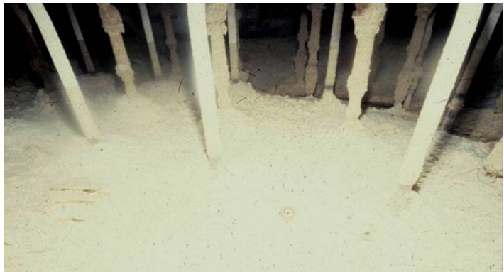
Figure 2.2-1: Saltcake at Bottom of Waste Tank
